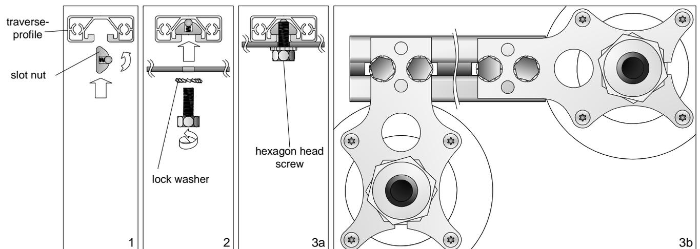
**Mounting of the sensor shelter TS at the mast fixation**
