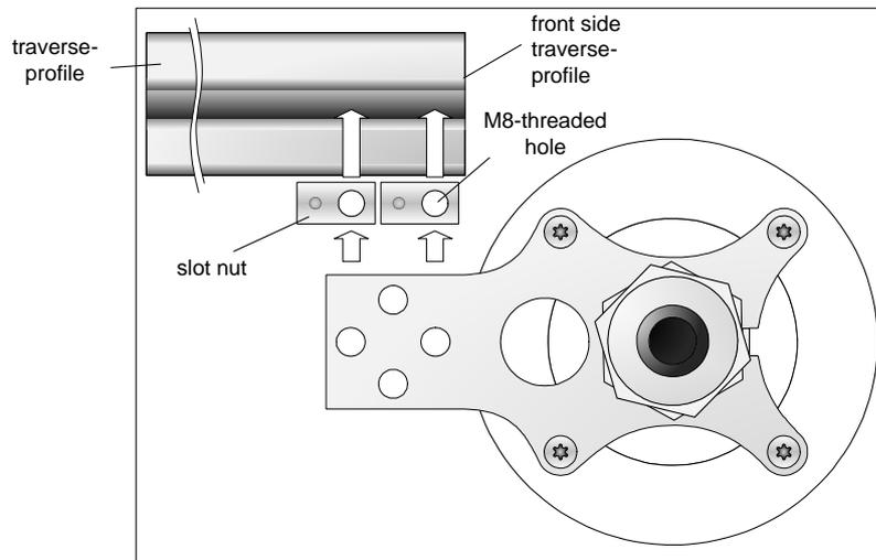
When inserting the slot nuts care must be taken to arrange the M8 threaded holes by pairs in line with the end of the traverse.
