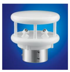
The ultrasonic wind sensor is designed without mechanical parts as they have been used with traditional "cups and vanes". The digital or analog output delivers instantaneous, average, min or max value with flexible measuring rate. The V200A-UMB is heated in case reaching critical ambient conditions.
