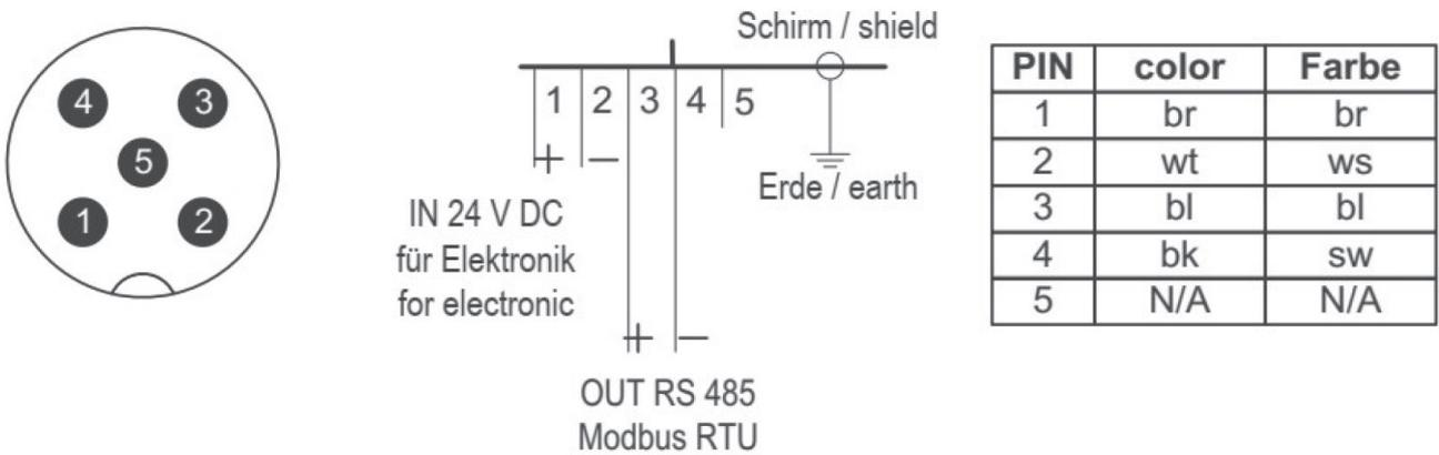
Cable-side socket (female) M12 4-pin, shielded
