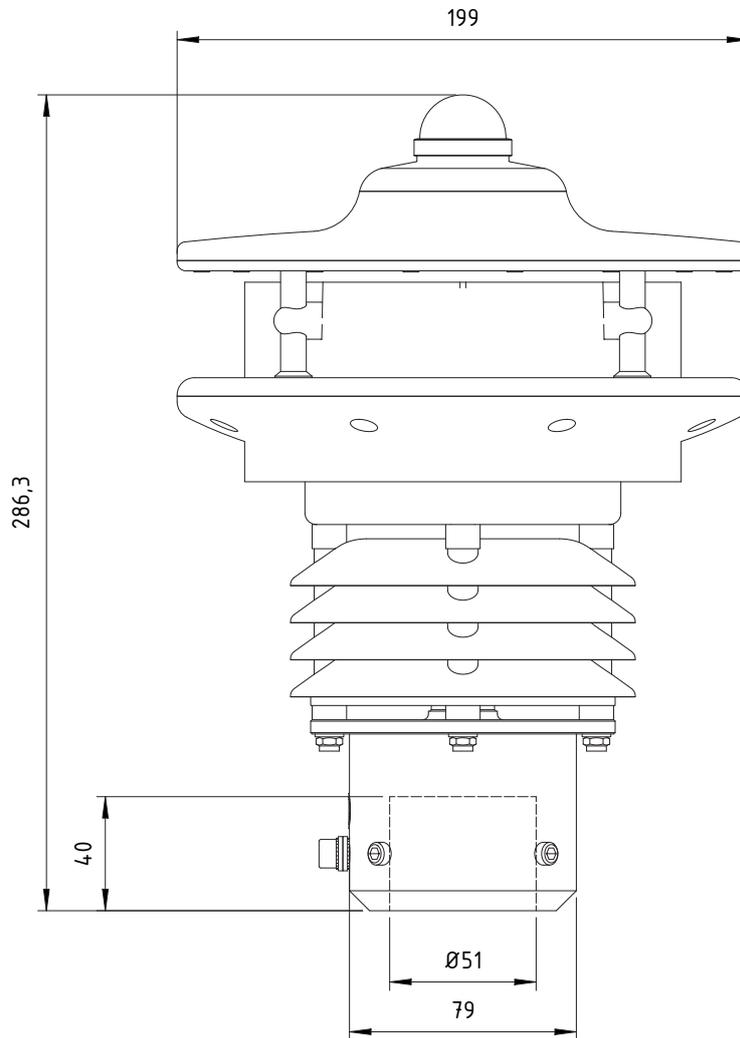
Sensor-side plug (male) M12 4-pin (or 5-pin), shielded
