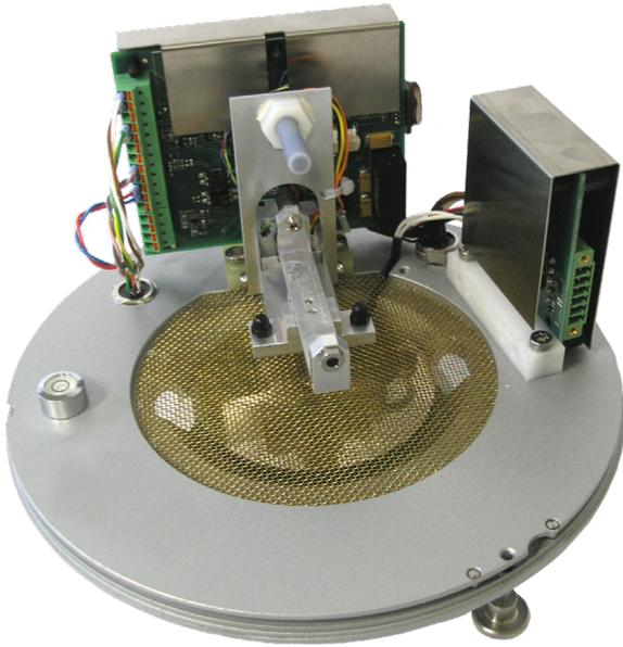
Inner workings of the **rain[e]** without collecting vessel.
