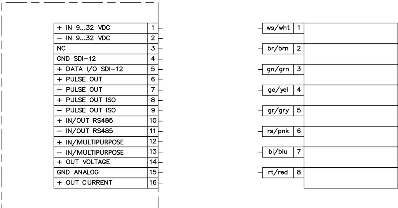
**Note:** The SDI-12 interface and the RS485 interface cannot be used simultaneously. Furthermore, it is recommended to apply only one of the two interfaces to the cable used at the same time.
