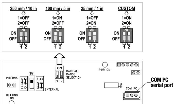
**Fig. 5 – Dip switches**
