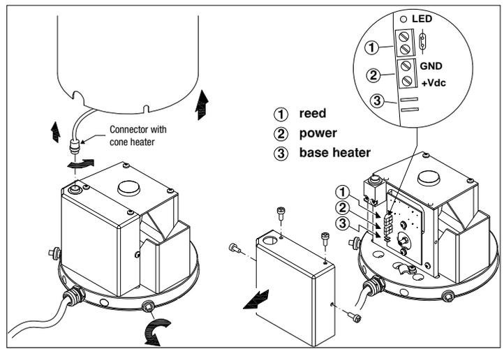
**Fig. 2 – Connections of contact output and heating**
