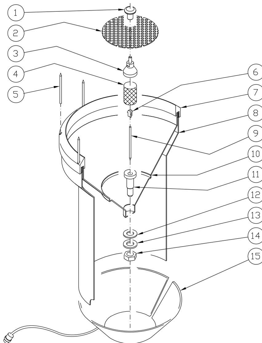
**Fig. 13 – Exploded view of the upper part (version with heating)**
