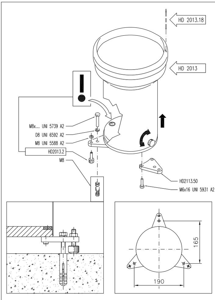
**Fig. 10 – Ground installation**
