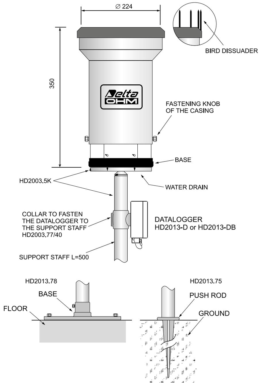
**Fig. 8 – Mechanical dimensions, installation modes**
