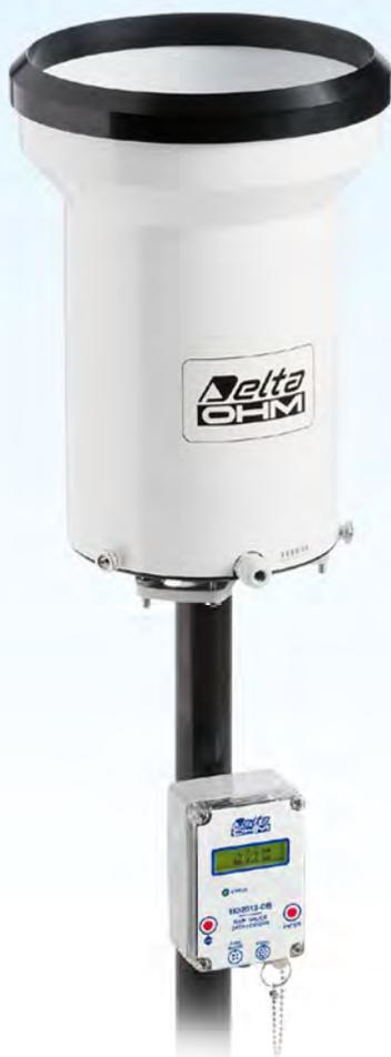
The HD2013 is a reliable and sturdy tipping bucket rain gauge, built entirely from corrosion resistant materials in order to guarantee its durability. So as to ensure accurate measurement even with low temperature climatic conditions or during and after precipitations of snow, a version with heating which is automatically activated around +4 °C has been developed so that snow deposits and ice formations are prevented.
