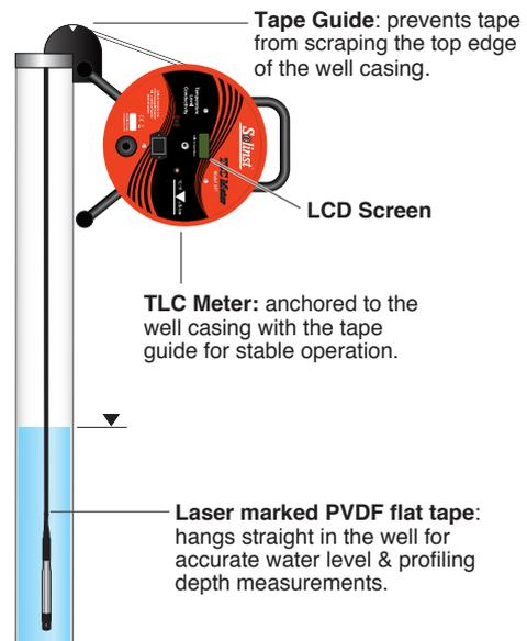
A Tape Guide/Datum allows the depth measurement to be read at the marked position on the Tape Guide, to give reliable, repeatable, accurate depth measurements when profiling a well. The Tape Guide protects the tape from damage on rough edges of well casing.
