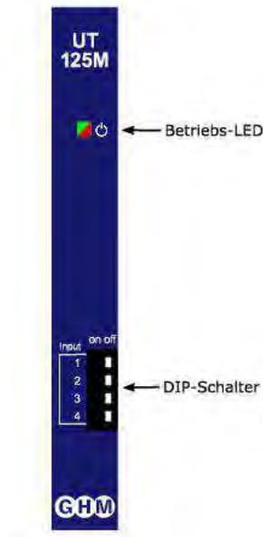
Selection of the measuring range takes place with DIP switches 1-4:
