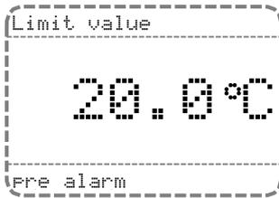
Alarm value (switching point) of the pre-alarm relay
