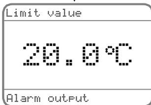
Limit value (switching point) alarm output
