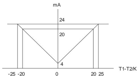
Characteristic curve B: The output signal is proportional to the difference  $T1-T2$ . The difference 0 Kelvin can be assigned to any desired current value in the range 4..20 mA, so that negative differences can also be represented.
