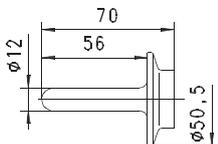
Sensor for Tri-clamp connection
