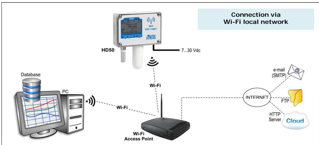
Multiple devices can be connected to the same local network, either via Wi-Fi (through a router or Wi-Fi access point) or via Ethernet. The data of all the devices connected to the network can be collected in the same database and can be viewed with a “Cloud” service, or can be downloaded via e-mail or FTP.
