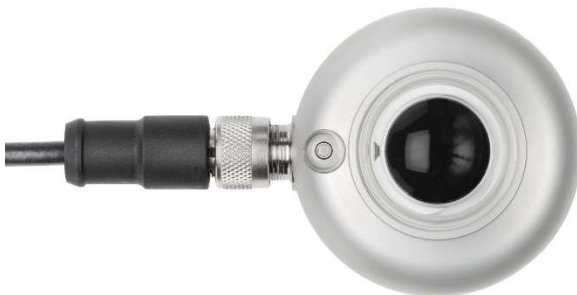
Figure 0.1 16103.5 second class pyranometer seen from above
