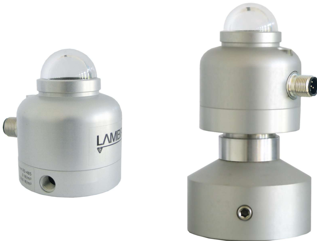
Figure 0.2 On the left 16103.5 second class pyranometer with bubble level and M12-A cable connector in its standard configuration; on the right 16103.5 with optional ball levelling 32.14627.006000, for easy mounting and levelling on the LAMBRECHT meteo traverse system 14627 and mast tube adapter 32.14567.006000.
