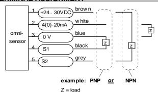
The switchpoints are changing to PNP or NPN depending to your Bitte benutzen interface automaticly. Please you use shielded cable, signal lines < 30m and power supply lines < 10m.
