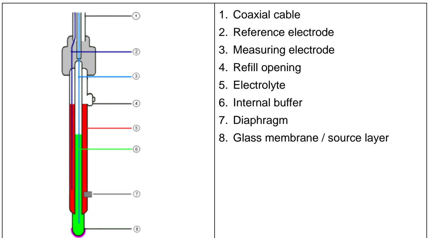
The diaphragm, which establishes a connection between the electrolyte and the liquid to be measured, can be designed in different ways. Clogging or soiling of the diaphragm is a frequent cause of a malfunctioning or sluggish electrode.
