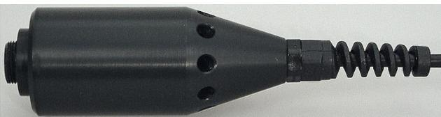
The sensor is equipped with drillings at the end and because of its special construction the measuring gas streams optimally around the sensor. No pressure can appear while gas blows to the sensor, which otherwise would result in erroneous measures. The temperature
