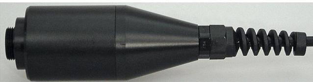
**For measurements at atmosphere** and in systems without over or under pressure the GGO... is sufficient. Additionally the GGO can be screwed tightly into systems with small over or under pressure. Attention! Mind the maximum pressure and the maximum
