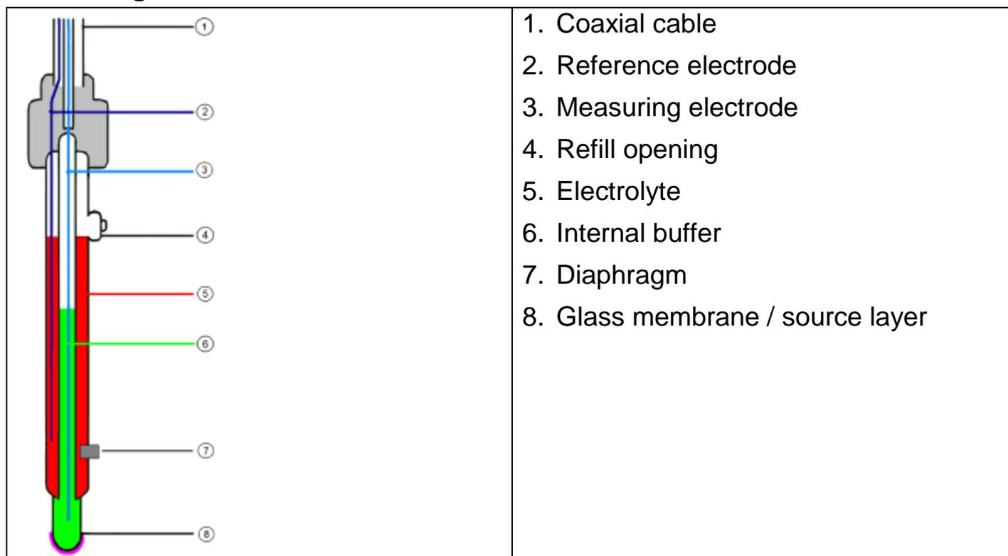
The diaphragm, which establishes a connection between the electrolyte and the liquid to be measured, can be designed in different ways. Clogging or soiling of the diaphragm is a frequent cause of a malfunctioning or sluggish electrode. Always
