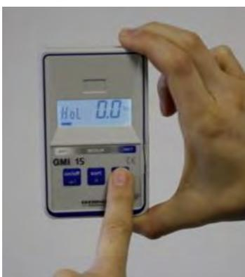
It is recommended to run regularly the zeroing function for best measuring results:
