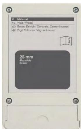
The entire grey surface has to lie on the measured material without any air gap.
