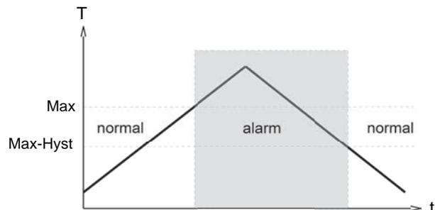
A changeover delay time ( $t_{DS}$ ) can be applied to switching to the alarm state. Equally, one switch-back delay time ( $t_{DR}$ ) of several can be applied to switching back to the normal state.
