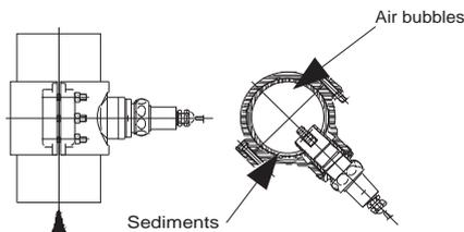
The best installation position (low contamination, good venting) is with the direction of flow from bottom to top, or in horizontal piping with the sensor at an angle of 45° downwards. The union nut must be tightened to a torque of 30 Nm.
