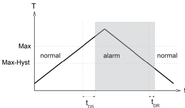
A changeover delay time ( $t_{DS}$ ) can be applied to switching to the alarm state. Equally, one switch-back delay time ( $t_{DR}$ ) of several can be applied to switching back to the normal state.
