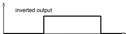
A Power-On delay function (ordered as a separate option) makes it possible to maintain the switching output in the normal state for a defined period after application of the supply voltage.
