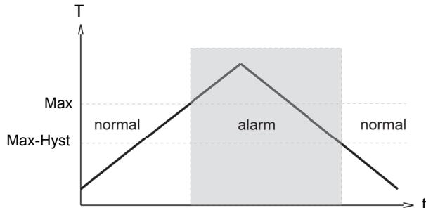
In the non-inverted (standard) model, while in the normal state the switching output is at the level of the supply voltage; in the alarm state it is at 0 V, so that a wire break would also display as an alarm state at the signal receiver. Optionally, an inverted switching output can also be provided, i.e. in the normal state the output is at 0 V, and in the alarm state it is at the level of the supply voltage.
