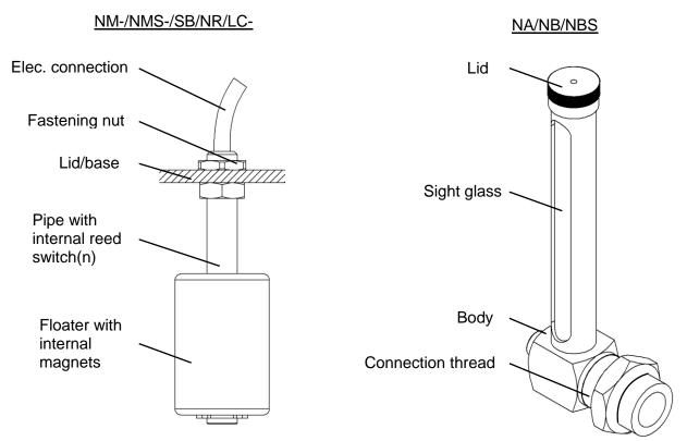
Figure 1: Schematic diagram of the devices NM-/NMS-/SB/NR/LC- and NA/NB/NBS
