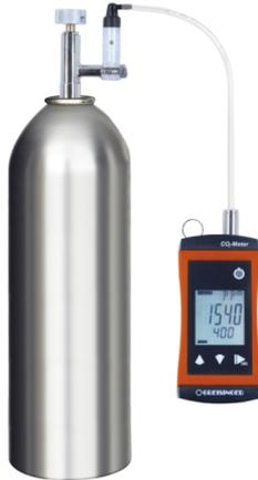
Calibration with test gas GZ-18 and adapter GZ-19
