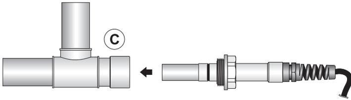
For direct connection of the probe, use a fitting with internal G 1/2" thread on the side which will be placed in the probe. The connection must be airtight. When installing or removing the model HP481, it is necessary to depressurize the system. Ensure that the probe does not obstruct the normal flow of air through the distribution line.
