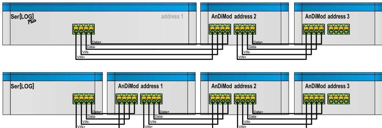
The Ser[LOG]Plus already contains an AnDiMod module (address 1) in its housing and can be extended by 2 additional AnDiMod up to 36 analog channels and 11 digital channels.
