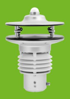
Seven meteorological parameters in one device
