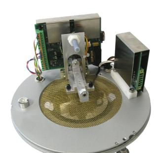
Inner workings of the **rain[e]** without collecting vessel.
