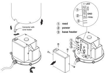
Fig. 3 – Electrical connections (version with heating option)
