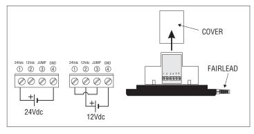
Fig. 1 Electrical connections
