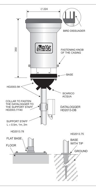
Fig. 2 Mechanical dimensions, installation systems
