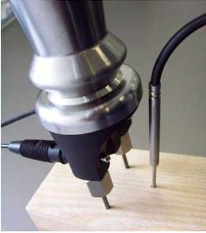
**Reciprocating piston electrode GHE91 with temperature-probe GTF38**
