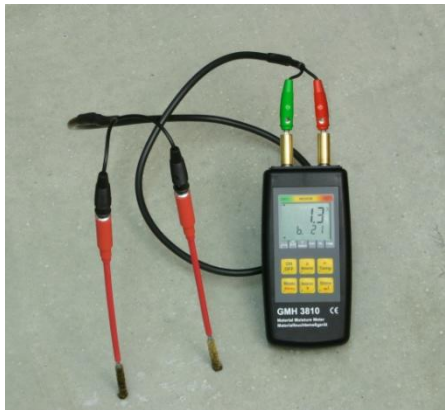
Measuring with brush probe GBSL91
