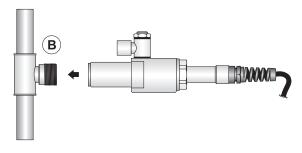
For the connection by threaded coupling, the connection must have an external G ¼" thread on the side which will be placed in the probe. The connection must be airtight. When installing or removing the probe, it is necessary to depressurize the system.
