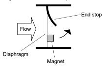
There is a plastic-coated magnet on the diaphragm. When there is a deflection, its magnetic field changes, and this is detected by a sensor outside the area of flow.
