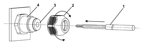
Figure 9: Connection PG-/cable screw gland
