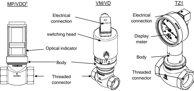
Figure 2: Schematic diagram for the devices MP/VDO, VM/VD and TZ1
