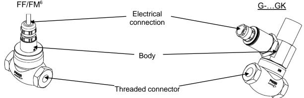
Figure 3: Schematic diagram for the devices FF/FM and G-...GK
