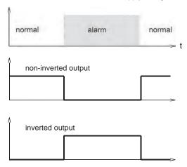
A Power-On-Delay function (ordered as a separate option) makes it possible to maintain the switching output in the normal state for a defined period after application of the supply voltage.
